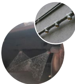
Custom made spray bar with dedicated nozzles for a conveyor
